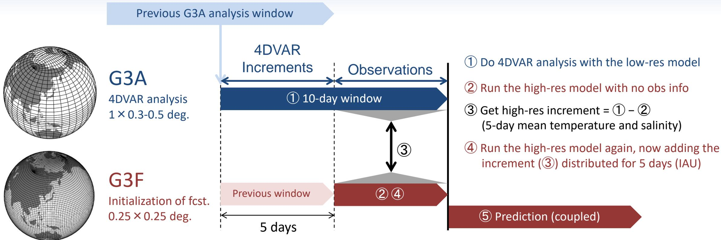
Experiments with a prototype system showed this setup outperforms straightforward 3DVAR with the 0.25-deg. model (with acceptable additional cost)
