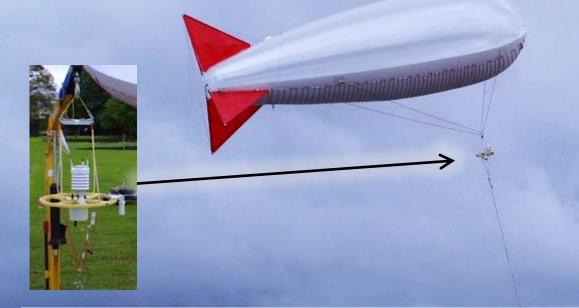
Pressure, Temperature, Humidity, Wind, Position(GPS), SST(infrared sensor) data is transferred every minute using IRIDIUM satellite communication system Flight duration :  $20 \sim 30$  days
