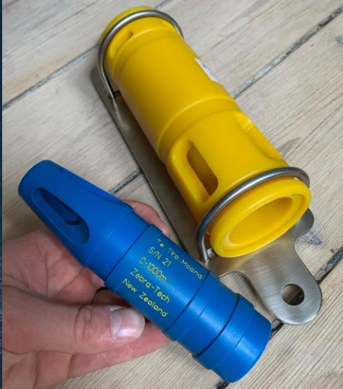
Zebra Tech Moana Profiling Temperature & Depth sensor with protective housing
