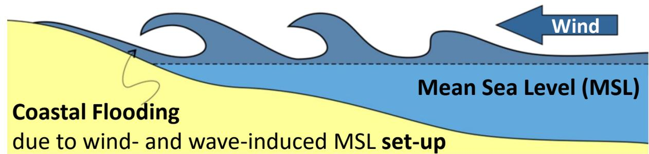
**Coastal Flooding** models include 3 approaches for coastal inundation due to Sea Level Rise
