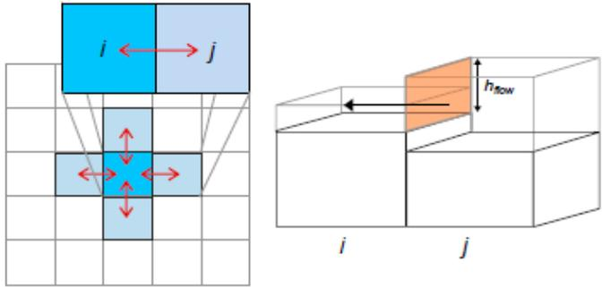
**Grid formulation:** treatment of water height over uneven bed elevation cells
