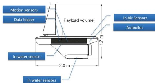
Figure 1: Sketch of the offshore sensing SailBuoy.
