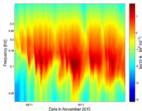
Figure 4: Spectrogram (power spectral density obtained from Waverider (1). The colour scale is logarithmic.
