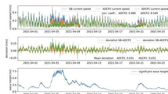
Figure 6: Depth-averaged current speed measured by the freely maneuvering SailBuoy ADCP and two moored reference ADCPs during an offshore test campaign. Deviation between the current speed measurements are shown in panel two. Panel three shows significant wave height data from a near-by weather station that affects the Sailbuoy's measurement capabilities (2).
