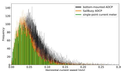
Figure 5: Histogram of the current speed data measured by the SailBuoy and bottom-mounted ADCPs and single-point current meter in Fusafjorden (inshore)(2).
