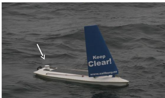
Figure 2: The offshore sensing SailBuoy.
